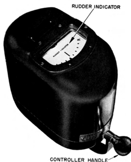
FIGURE 46. Non-Follow-Up Controller with Rudder Angle Indicator.
