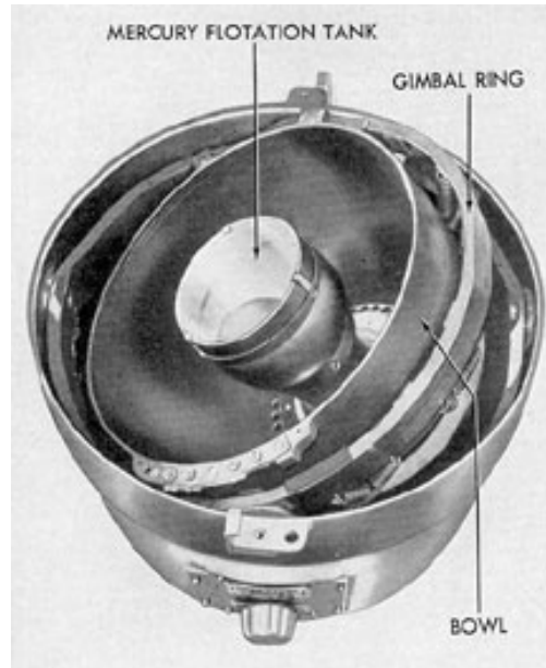
Figure 17-38. Arma auxiliary gyrocompass Mark 9, lower housing, gimbals and mercury flotation tank.
