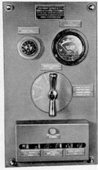
Figure 17-40. Arma auxiliary gyrocompass Mark 9 control panel.
