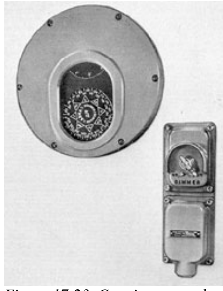
Figure 17-23. Conning tower double dial steering unit with dimmer switch.
