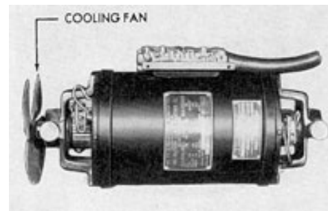
Figure 17-39. Arma auxiliary gyrocompass Mark 9 motor generator set with end covers removed.
