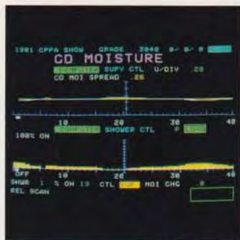
Measurex Total Profile Control provides precise cross-direction control of all three
