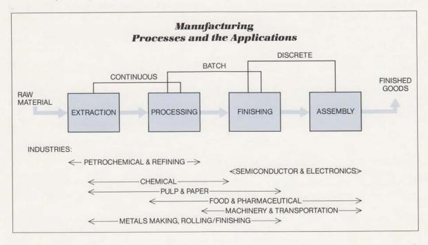
As shown in the illustration on Page 4 (in blue), the raw material input goes through a variety of applications, starting with extraction, before it comes out as a finished product. Each application involves one or a combination of manufacturing processes, whether it be continuous, batch or discrete. As a result, many companies require controls for continuous, batch and discrete manufacturing processes all at the same plant, integrated into a plantwide information system.
