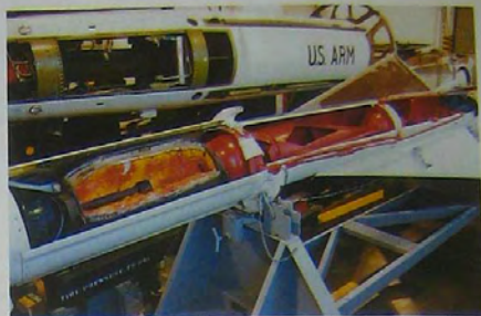
Ajax, from left: green guidance, yellow forward High Explosive (HE), red hypergolic tank. Hercules sustainer in background. (Wilson, Meyerriecks)
