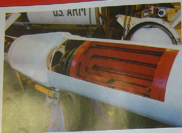
Nike solid propellant grain. Note nine port extruded grain for a very neutral thrust profile, and resonance rods in each port to improve combustion stability. (Meyerriecks)
