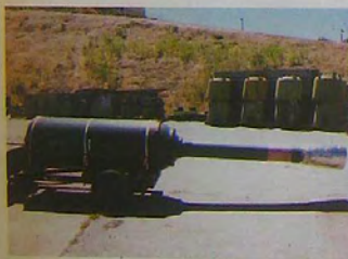
Hercules solid propellant sustainer, Nike Hercules interstage adapters background. Note the exceptionally long throat! (Meyerriecks)
