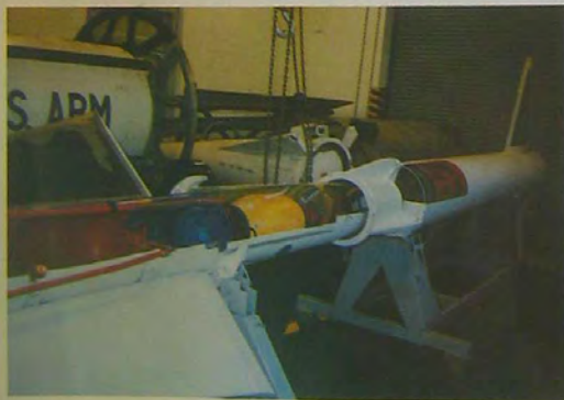
Nike Ajax: red hypergolic fuel tank, blue pressurized nitrogen tank, yellow aft HE, red combustion chamber/nozzle (in interstage). Note Ajax 'honeycomb' fin and Hercules guidance/warhead section in background in left photo. Nike front end/interstage (right). Red double-base grain held in place by forward spring. (Wilson)
