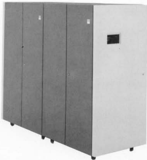
The photo of a design model shows: one 'A' box (with operator panel) one 'B' box (3 boxes are possible)
